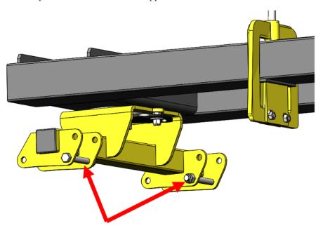
Install 0.625" x 5" bolts (2 pcs) and 0.625" nyloc nuts (2 pcs) in the locations shown. Only tighten enough to keep the bolts from rotating on their own. Use 2pcs 15/16" wrenches.
