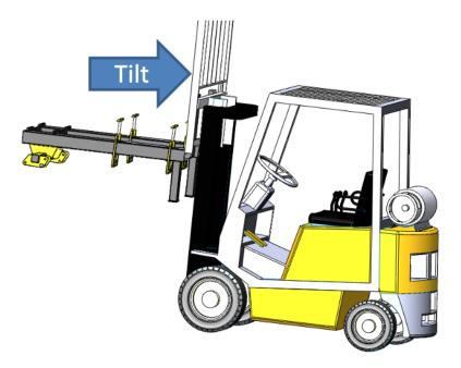
Lift up the fork pocket assembly with forklift. Make sure the forks are tilted backwards so the assembly won't slide off of the forks.
