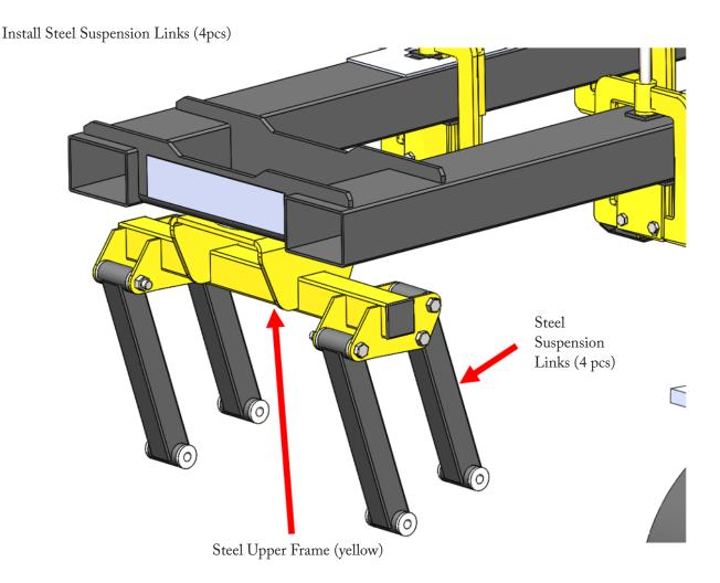
Install the Steel Suspension Links (4pcs) in the remaining 4 hole locations in the Steel Upper Frame using 4x 0.625" x 5" bolts (4pcs) and 0.625" nyloc nuts (4pcs).
