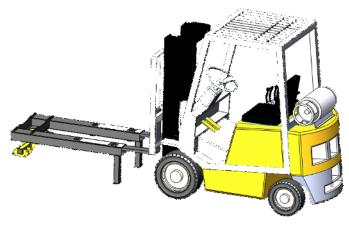
Remove Fork Pocket Assembly from Pallet with Forklift.
