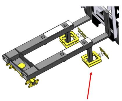
Set the four Fork Clamp Assemblies on the Ground (two around each Parking Stand) as shown and lower the Fork Pocket Assembly down to the ground with the fork lift.
