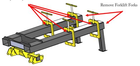
Move Clamp Assemblies into Position as shown by lifting them up the parking stands and flipping them around the tubes where the forks were removed until they are each in position.
